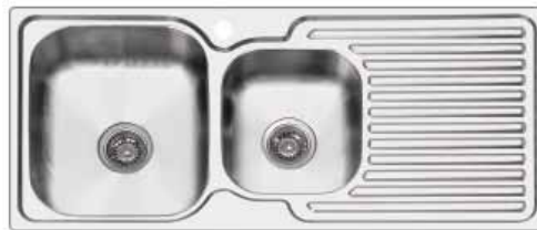
AB.PR175R.SS (Right hand bowl) AB.PR175L.SS (Left hand bowl) Project 175 - One & Three Quarter Bowl Overall Sink Size: 1080mm L x 480mm W Bowl Sizes: 355mm L x 405mm W x 165mm D, 280mm L x 310mm W x 160mm D
